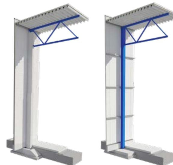
Reinforced concrete column with truss beams
